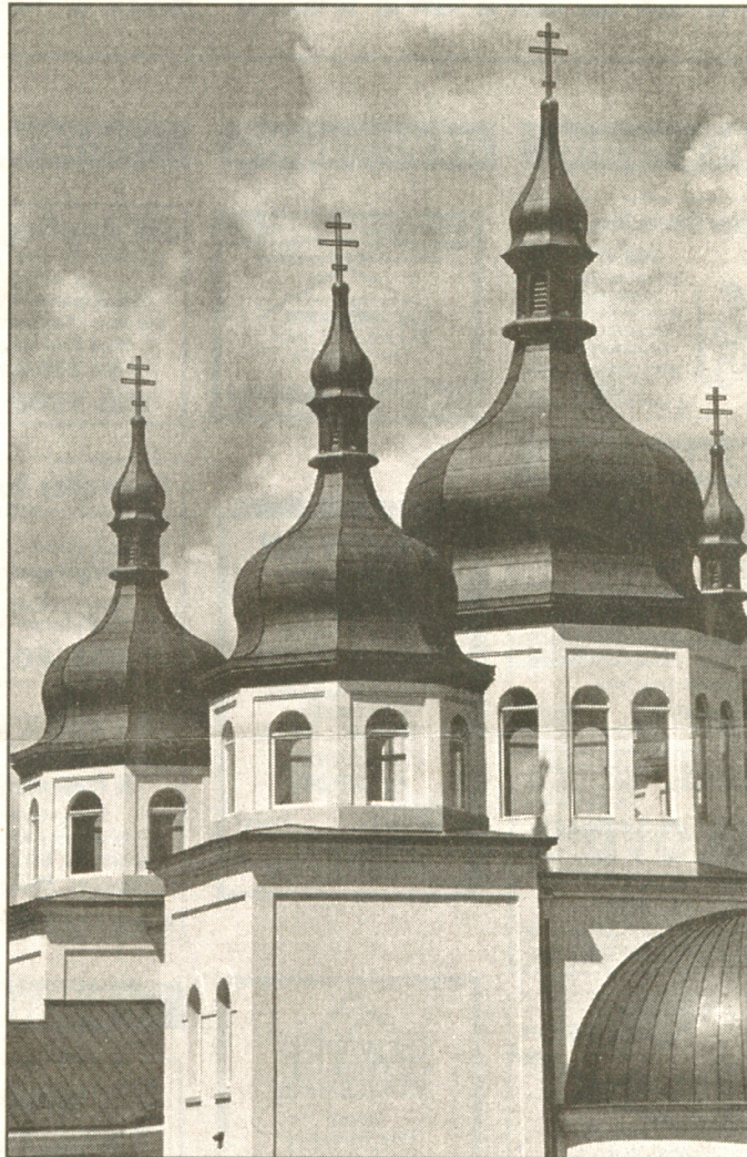
The five copper domes are visible from Highway 96. But the rest of the Ukrainian Baroque architectural style is better seen upon closer inspection. What visitors will see is an exterior of white stucco walls with precast artstone trim and arch head design windows. (Photo by Paul Dols)
